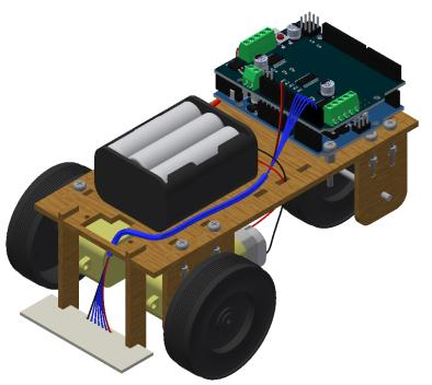
14. Connect the battery pack to the motor shield using the 9v battery connector. The red wire goes to the M+ terminal and the black wire goes to the GND terminal.
