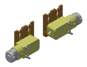
3. Attach the motor and axle mounts to the base plate using the 20mm screws:
