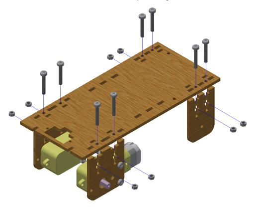
**NOTE**: **Do not over tighten the screws**. Acrylic is a very brittle plastic and will crack easily if too much force is applied. Don't worry if the mounts have a little bit of movement in them, this will not affect the robot's functionality.
